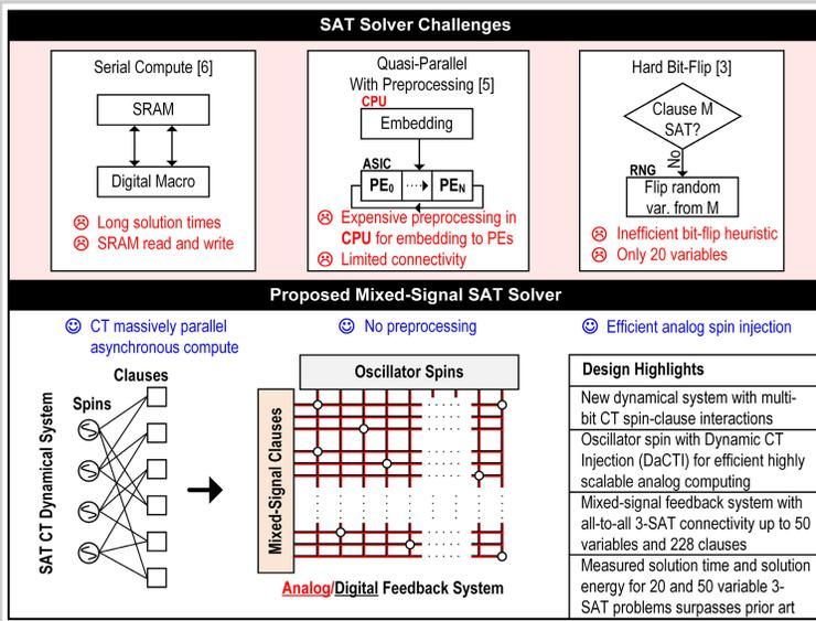
Figure 25.1.1: Overview of recent Boolean satisfiability (SAT) solver architectures and their limitations. Introduction to the proposed mixed-signal SAT solver and design highlights.
