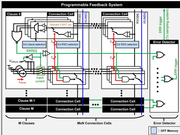
Figure 25.1.3: Crossbar-based spin feedback architecture. Current summation line (ISUM) architecture with TIA and pre-charge improves delay.
