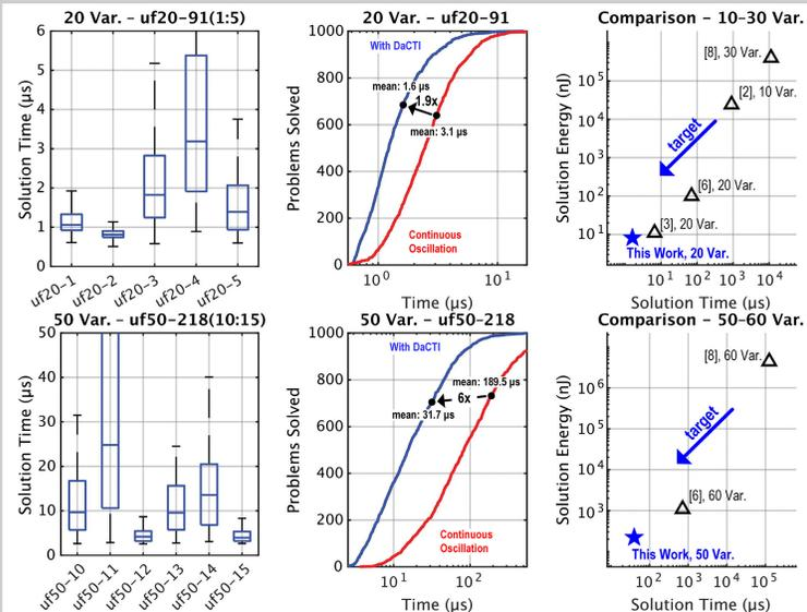
Figure 25.1.5: Measured results for 3-SAT problems with 20 variables/91 clauses and 50 variables/218 clauses from the SATLIB benchmark. Solution time distribution of instances and cumulative results for all benchmark problems. Prior art comparison.
