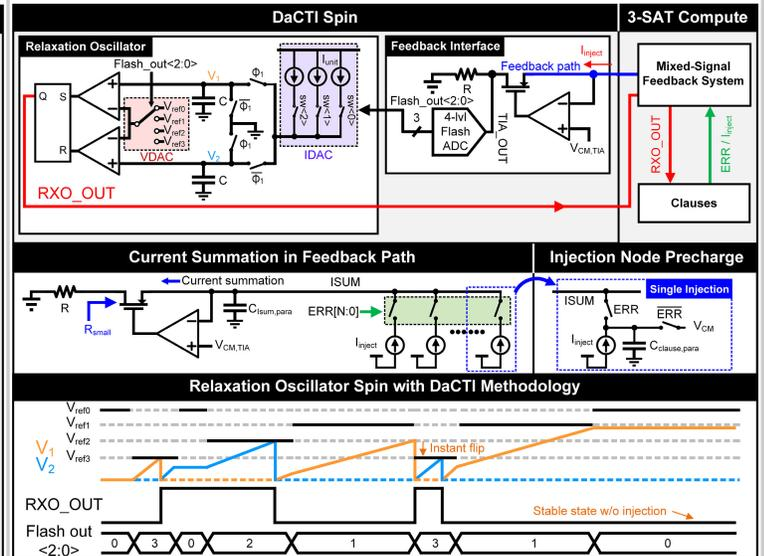
Figure 25.1.4: Relaxation-oscillator-based spin with Dynamic CT Injection (DaCTI). Current summation architecture and DaCTI timing diagram.
