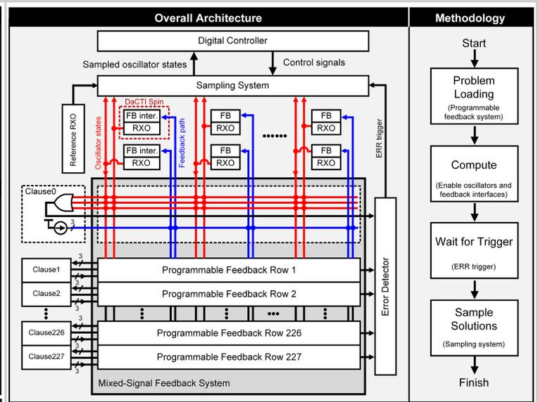
Figure 25.1.2: Proposed solver architecture with key design blocks and methodology.
